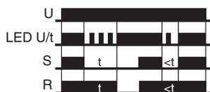
contact S is closed, the output relay R switches into on-position (yellow LED illuminated). If the control contact S is opened, the set interval t begins (green LED U/t flashes). After the interval t has expired (green LED U/t illuminated) the output relay switches into off-position (yellow LED not illuminated). If the control contact is closed again before the interval t (green LED U/t illuminated) has expired, the interval already expired is erased and is restarted with the next cycle.
