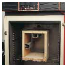
Cabin for age acceleration test.
