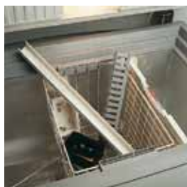
Refrigerator to prepare samples for low temperature shock tests.
